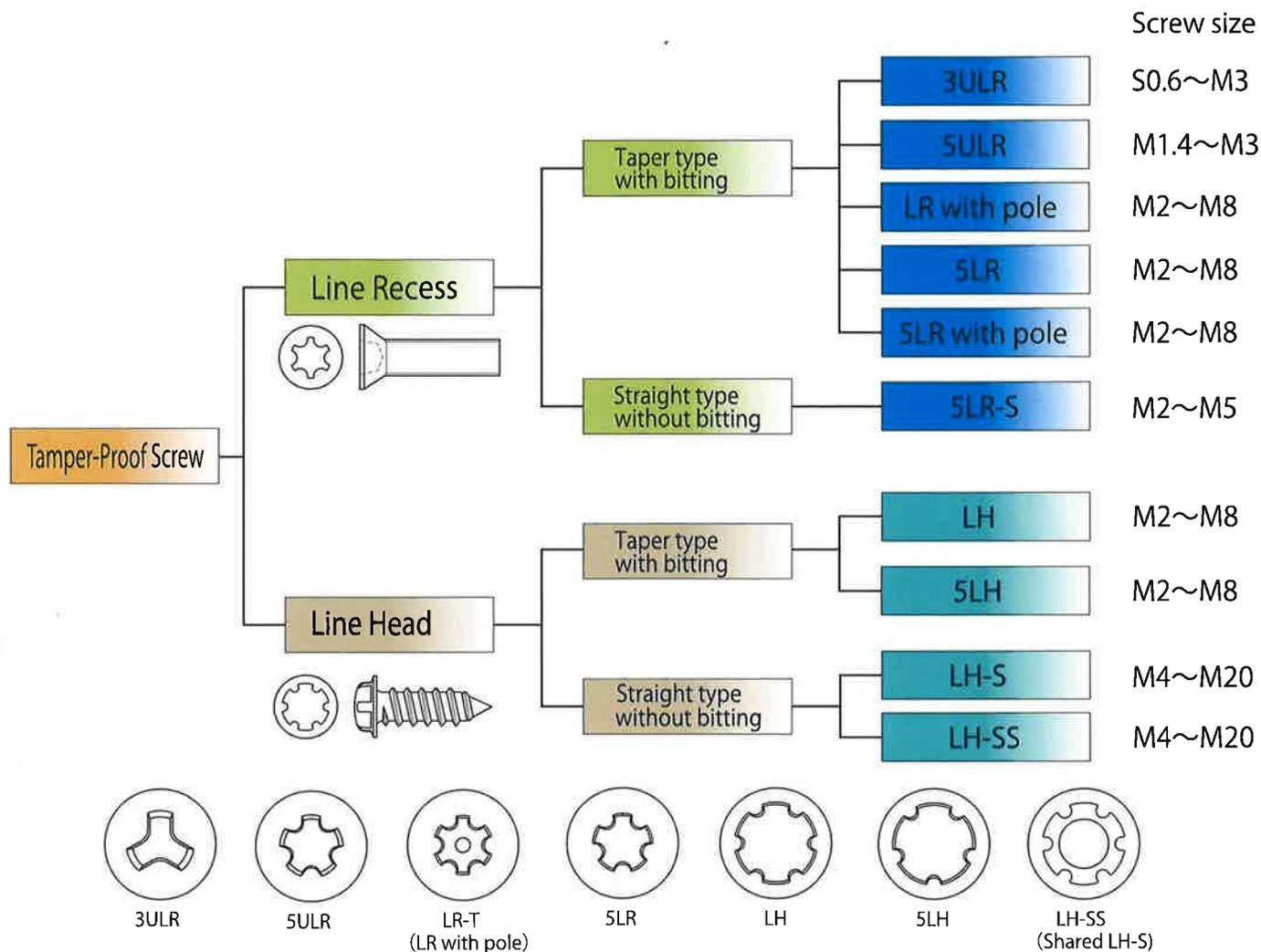
※ Available with tapping screws and the other standard screws can be adaptable.
